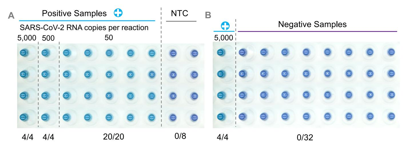
The assay was carried out using either positive samples (human total RNA plus synthetic SARS-CoV-2 RNA at 5,000, 500 or 50 copies per reaction), negative samples (human total RNA alone) or no template (NTCs), as indicated. The 25 µl reactions were incubated at 65°C for 45 minutes, cooled to room temperature and then visually inspected.
