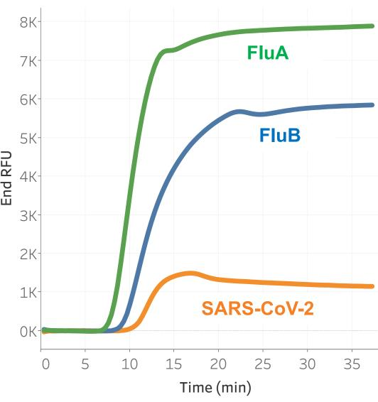
TaqMan-like hybridization probes are easy to design and have been shown to be effective in LAMP/RTreactions.<sup>3</sup> Compatibility of the lyophilized LAMP/RT-LAMP Mix (no dye) was evaluated using previously designed probes for three common respiratory RNA viruses: FluA (Cy5), FluB (FAM) and SARS-CoV-2 (HEX).
