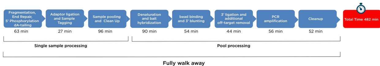
**Figure 1.** The complete workflow of the NEBNext Direct Genotyping Solution. Indicated below each process is the duration of the individual steps for the processing of 96 samples using 96 pre-capture sample indexes and 1 post-capture pool index.
